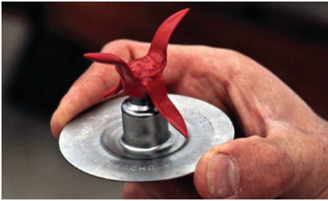
Figure 8.17 —Modifying kitchen blender blades by using rubber coating allows the grower to clean small lots of dry and fleshy fruits without damaging the seeds. Photo by R. Kasten Dumroese.
