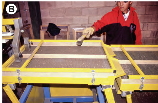
Figure 8.13 —Screens are used to separate large debris and fine chaff from the seeds and are available commercially in a wide range of screen holes sizes to compliment any species (A). Seeds of many species are very small and require fine screens or sieves for cleaning (B). Photo A by Tara Luna, and photo B by Thomas D. Landis.
