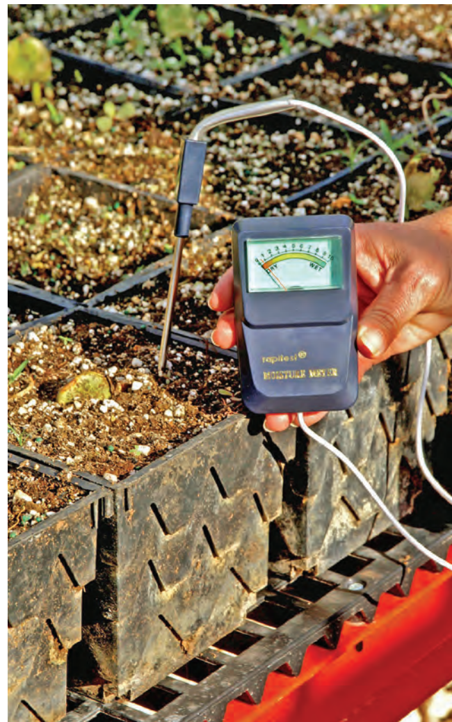
Figure 11.14 —Many types of tools can be used to help test and assess the effectiveness of water application, including this moisture meter. Visual and tactile assessments are more prevalent in tropical plant nurseries, however, and can be quite effective when carried out by trained staff. Photo by Thomas D. Landis.
