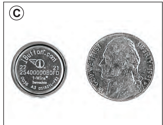
Figure 5.13 —Monitoring and controlling temperature is critical to successfully growing a crop of tropical plants (A). Many nurseries use small, programmable, self-contained temperature sensors that record daily maximum and minimum temperatures (B and C). Photo A by Thomas D. Landis, and photos B and C by David E. Steinfeld.
