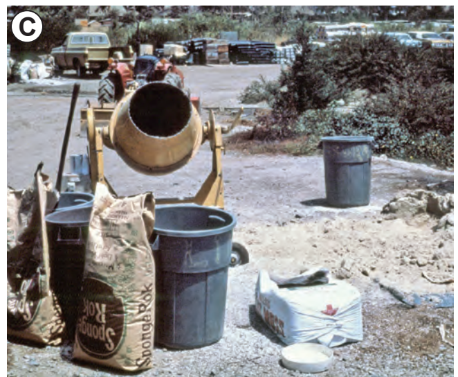
Figure 6.14 —Nurseries that mix their own media can do so by hand (A) or by using the moving pile technique (B). To reduce labor, a cement mixer (C) can also be used but care must be taken to avoid overmixing and resultant damage to particle size and structure. Photo A by Diane L. Haase, and photos B and C by Thomas D. Landis.
