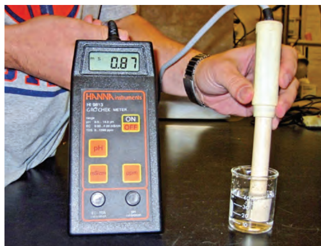
Figure 12.15 —An electrical conductivity meter used to estimate fertilizer salt concentrations in irrigation water, fertigation water, or saturated media extract. Photo by Douglass F. Jacobs.
