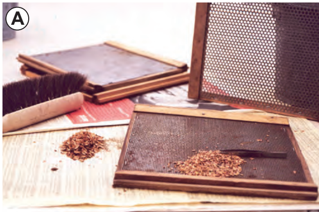
Figure 8.13 —Screens are used to separate large debris and fine chaff from the seeds and are available commercially in a wide range of screen holes sizes to compliment any species (A). Seeds of many species are very small and require fine screens or sieves for cleaning (B). Photo A by Tara Luna, and photo B by Thomas D. Landis.
