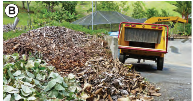
Figure 16.3 —Culled seedlings, old growing media, and other greenhouse waste can be composted (A). Woody materials and other green waste can be ground into smaller pieces by machinery to speed-up the composting process, as shown here at the nursery at Parque Doña Inés in San Juan, Puerto Rico (B). Photos by Brian F. Daley.
