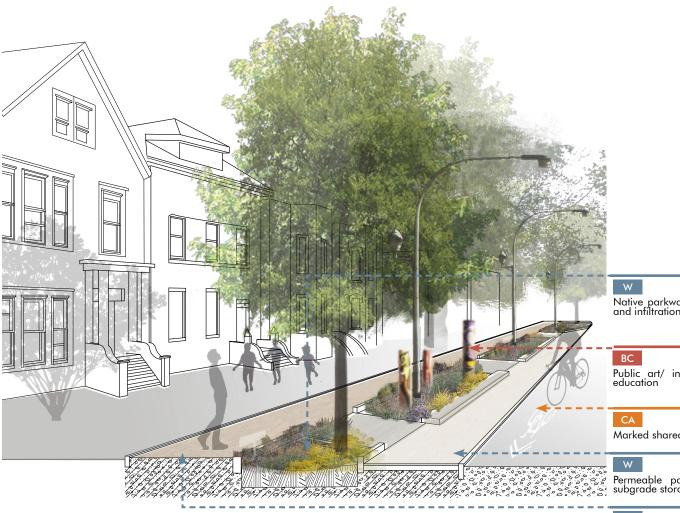
Native parkway bioswale (captures stormwater for storage and infiltration)
