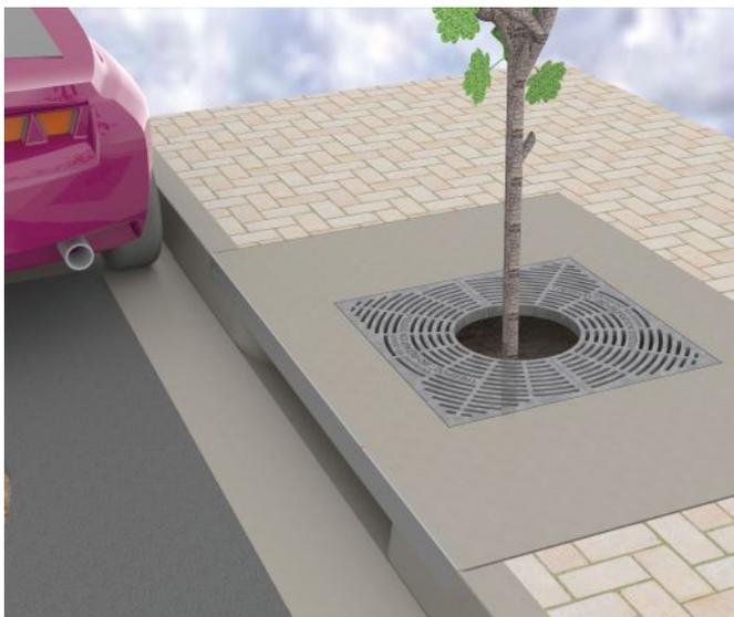
ment system, the city selected TreePod biofilters manufactured by Oldcastle Stormwater. TreePod biofilters are open-bottomed box filters that remove suspended solids, petrochemicals,
